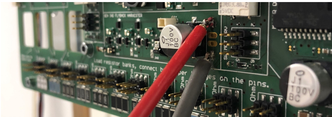
Figure 14: Probes to measure harvested electrical energy.
