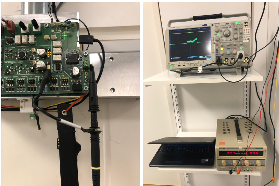
Figure 15: Setup to measure energy required for automatic opening.
